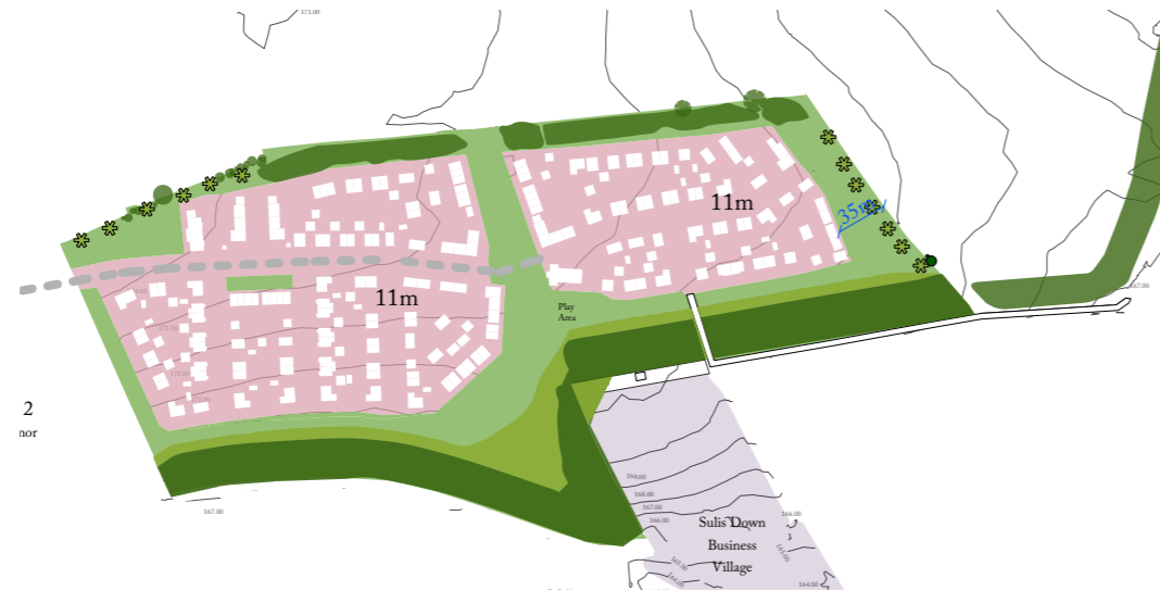
Scenario 5: Retention of northern boundary Extension and strengthening of southern boundary Developable area pulled back from eastern boundary by 35m 11m max height parameter
