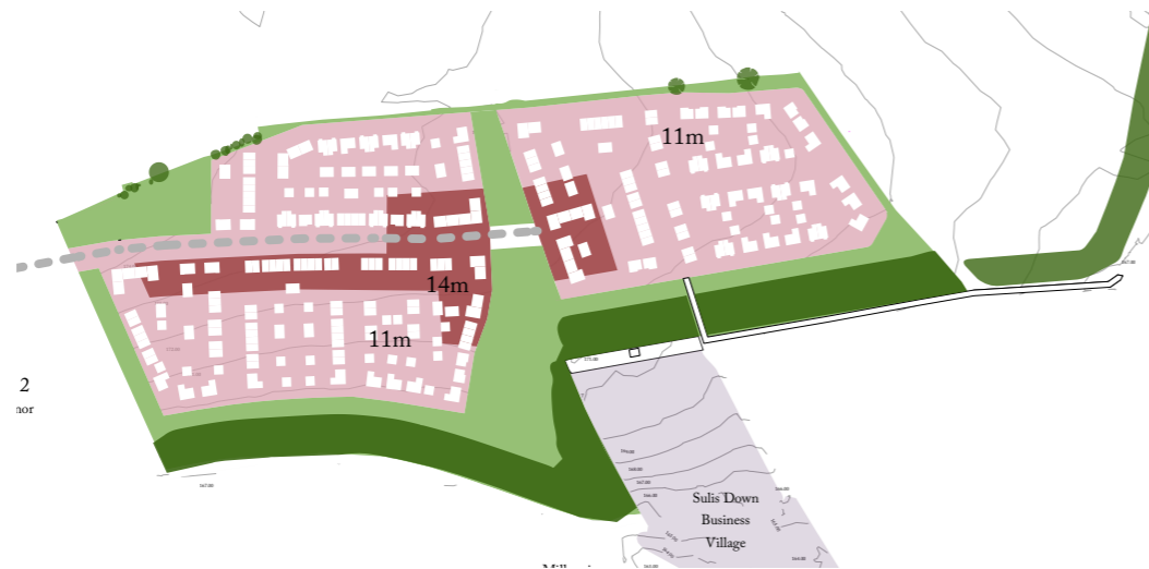
Scenario 1: Appeal Scheme Northern boundary vegetation removed, No additional woodland, 14m max height parameter Developable area extending to eastern boundary, 290 homes
